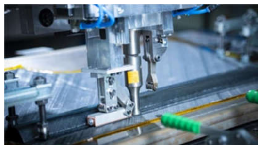
Fig. 2: Welding of omega-stringer with continuous Ultrasonic Welding (cUW)
