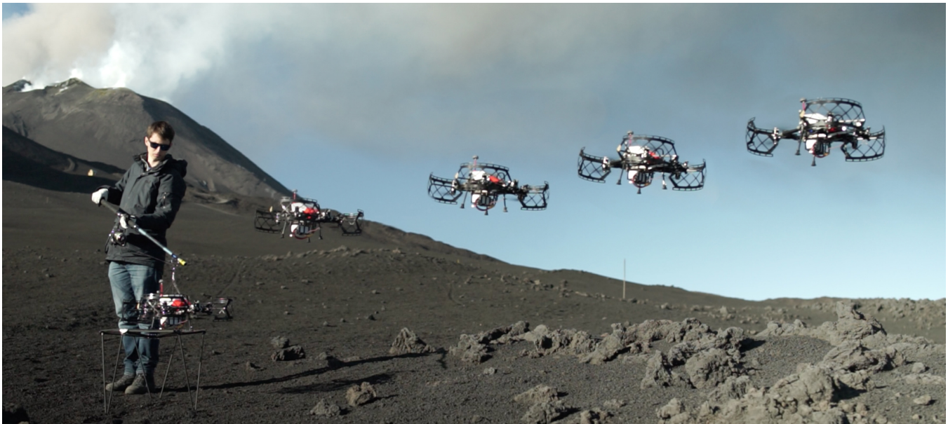
Figure 18. ARDEA using the proposed terrain following on Mt. Etna. The person in the image is holding a safety tether, which is just used for emergency cases. The person is removed in parts of the image for better visualization.
