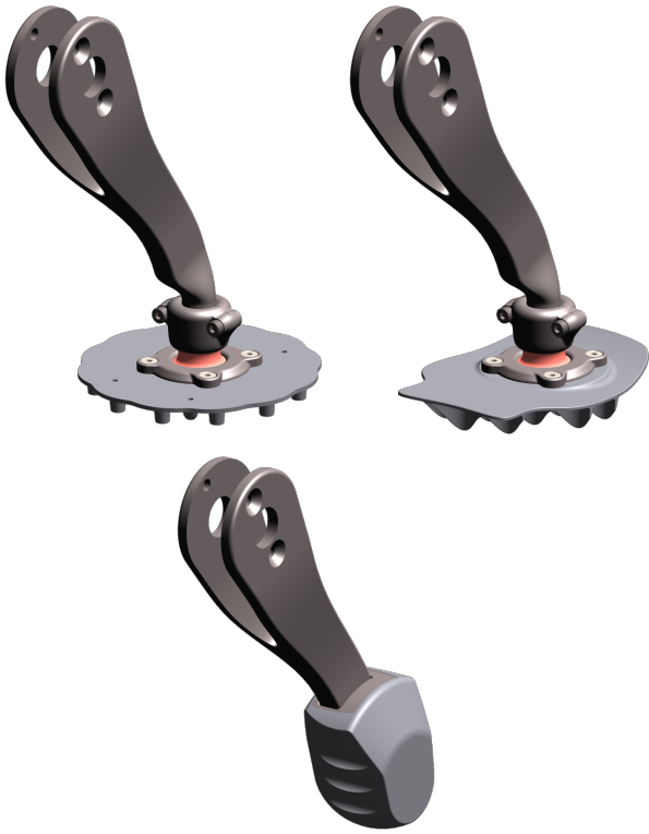
Figure 6. CAD model of the different feet. The upper two feet use a passive planar joint with different contact plate designs. The first contact plate is circular shaped and equipped with simple spikes (top left), the second plate features a pattern of small shovels at the bottom and a forward displaced force transmission point (top right). The foot displayed at the bottom is the regular rubber point foot normally used for normal conditions on flat surface.
