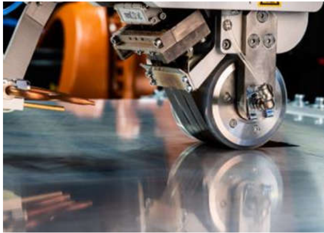
Incoming tapes, laying at a heated tooling
