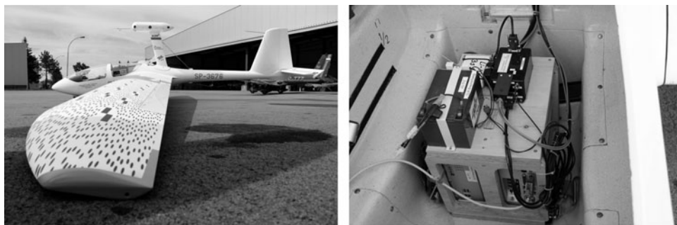
Figure 5. Dot pattern and markers on the wing (left) and recording hardware stored in the rear cabin (right).
