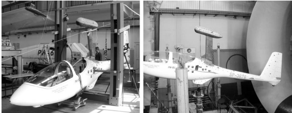
Figure 6. Static tests (left) and wind tunnel tests (right) were performed to prove the stiffness, strength and stability of the camera pod.
