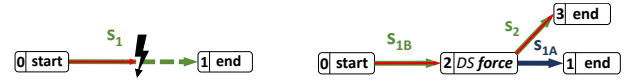
(c) The robot stops the execution of skill s_1 at the timestep of an anomaly detection.
