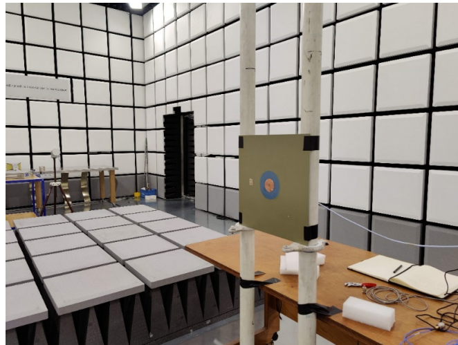
Figure 6: Measuring setup used in measuring the radiation pattern of the antenna demonstrator. A Right Handed Circular Polarized (RHCP) antenna or a Left Handed Circular Polarized (LHCP) antenna is placed on the far side of the room. The antenna demonstrator is rotated from -90 to 90 degrees.
