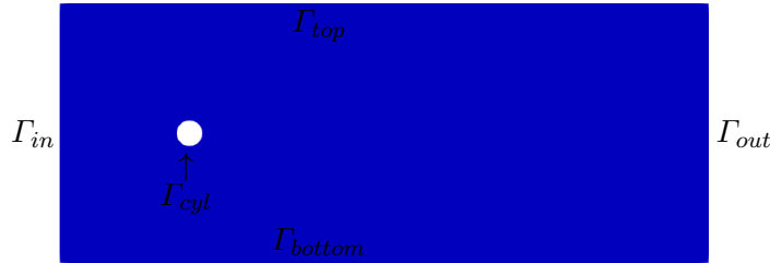
FIGURE 4.1: Physical domain of the CFD test case. The cylinder is depicted in white, the fluid domain in blue.
