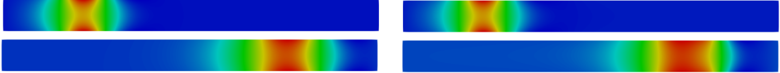
FIGURE 4.13: Pressure snapshots (left column) at time t = 0.005 (top) and final time t = 0.015 (bottom). Reduced order pressure simulation (right column) at time t = 0.005 and time t = 0.015 . The reduced simulation has been obtained with N = 4 basis functions, for each component of the solution of the FSI problem.
