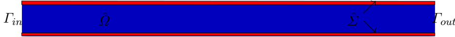
FIGURE 4.6: Physical domain (reference configuration): fluid subdomain (blue) and structure subdomain (red). The fluid-structure interface coincides with the structure in our case; the structure has been magnified for visualization purposes.
