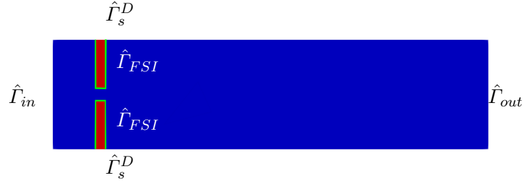
FIGURE 3.1: Physical reference configuration. Blue domain: the reference fluid configuration \hat{\Omega}_f . Red leaflets: the reference solid configuration \hat{\Omega}_s . The fluid–structure interface \hat{\Gamma}_{FSI} is depicted in green. \hat{\Gamma}_s^D : the part of the leaflets that does not move.
