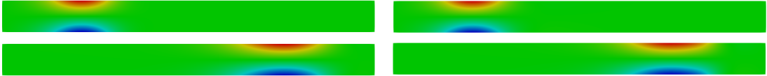
FIGURE 4.14: Displacement snapshots (left column) at time t = 0.005 (top) and final time t = 0.015 (bottom). Reduced order displacement simulation (right column) at time t = 0.005 and time t = 0.015 . The reduced simulation has been obtained with N = 4 basis functions, for each component of the solution of the FSI problem.
