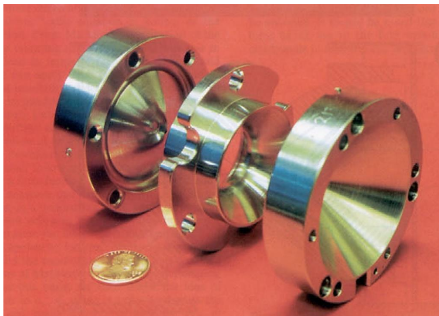
Figure 5 Diagram of the two endcap electrodes and ring electrode in a quadrupole ion trap. Reprinted with permission from John Wiley and Sons. In Journal of Mass Spectrometry, An Introduction to Quadrupole Ion Trap Mass Spectrometry , Raymond E. March. Copyright 1998.
