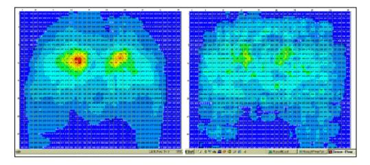
*Note*. Pressure mapping visual comparison. Cushion on left presents with high pressure points, while cushion on right presents with low pressure point, and improved pressure distribution (University of Washington, 2004).
