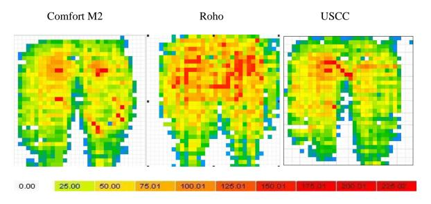
*Note:* Visual representation of pressure sensor readings through a white (low pressure) to red (high pressure) color gradient.
