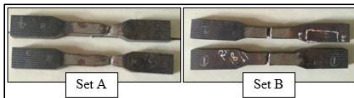
Figure 4: Fracture line from the Tensile Test
