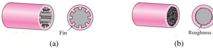
Figure 4: Tube surface (a) finned surface and (b) roughened [18]
