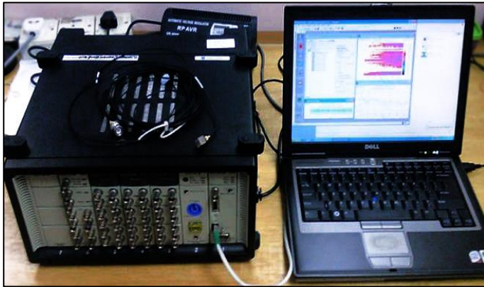
Figure 8: The Bruel & Kjaer PULSE™ Multi-Analyzer System connects to a computer with PULSE LabShop software.
