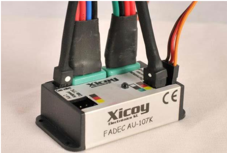
Figure 8: Ports on FADEC ECU
