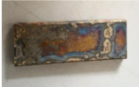
Figure 4: Ti6Al4V Surface condition after the heat treatment process in water quenching medium.
