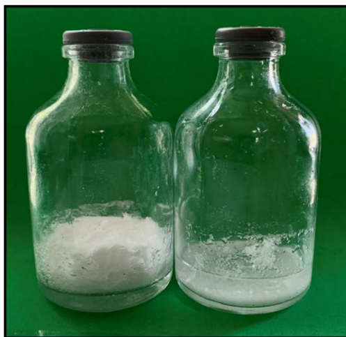
Figure 4-1 Representation of collapse in typical freeze-drying samples. (Left) Partially collapsed and (right) fully collapsed/melt-back samples.
