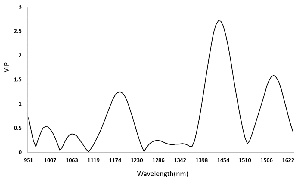
Figure 3-10. PLS VIP. Wavelengths with values >1 are considered important for predicting moisture.
