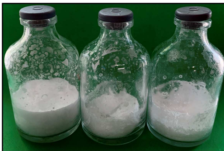
Figure 4-2 Representation of typical finished freeze-dried samples. (Left) Normal cake, (center) partially collapsed, and (right) fully collapsed/melt-back samples.
