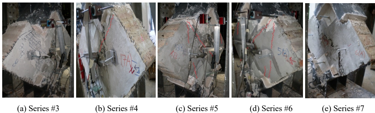
Fig. 11 Appearances of the failure mechanisms of the strengthened masonry walls
