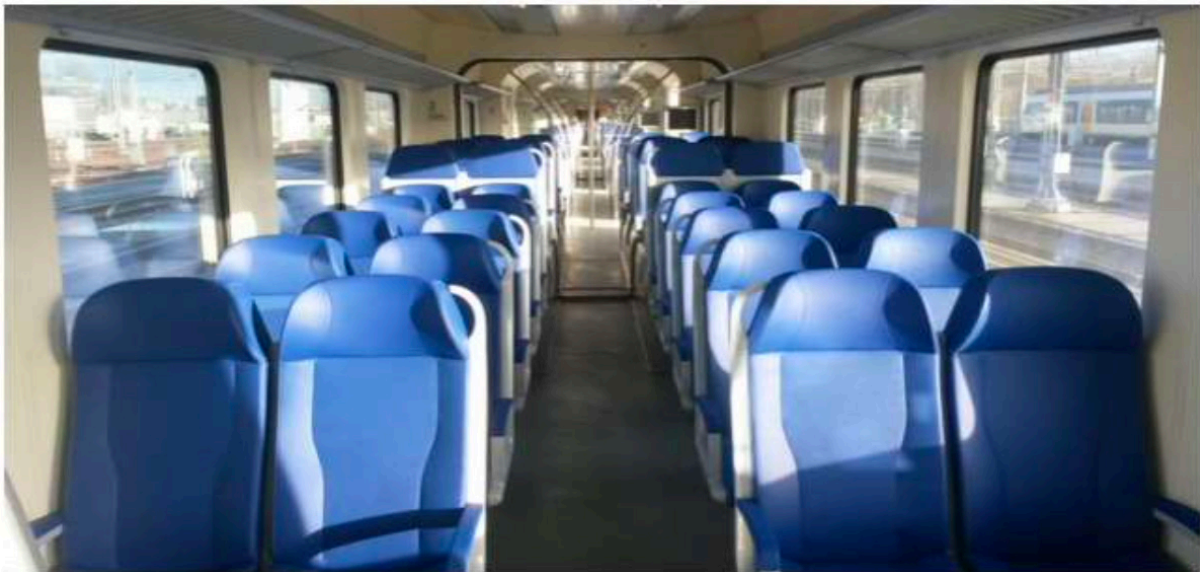
Figure 1 Photo of the train compartment with (smooth) vinyl seating materials.
