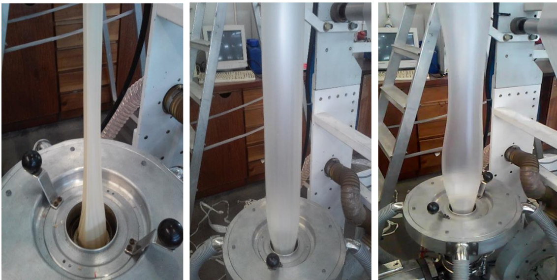
Figure 1. Preliminary film blowing trials with PHB (left) and PHB modified by DCP (middle and right).
