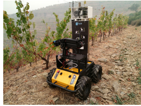
Fig. 6. The AgRob V16 agriculture robot monitoring a slope vineyard.
