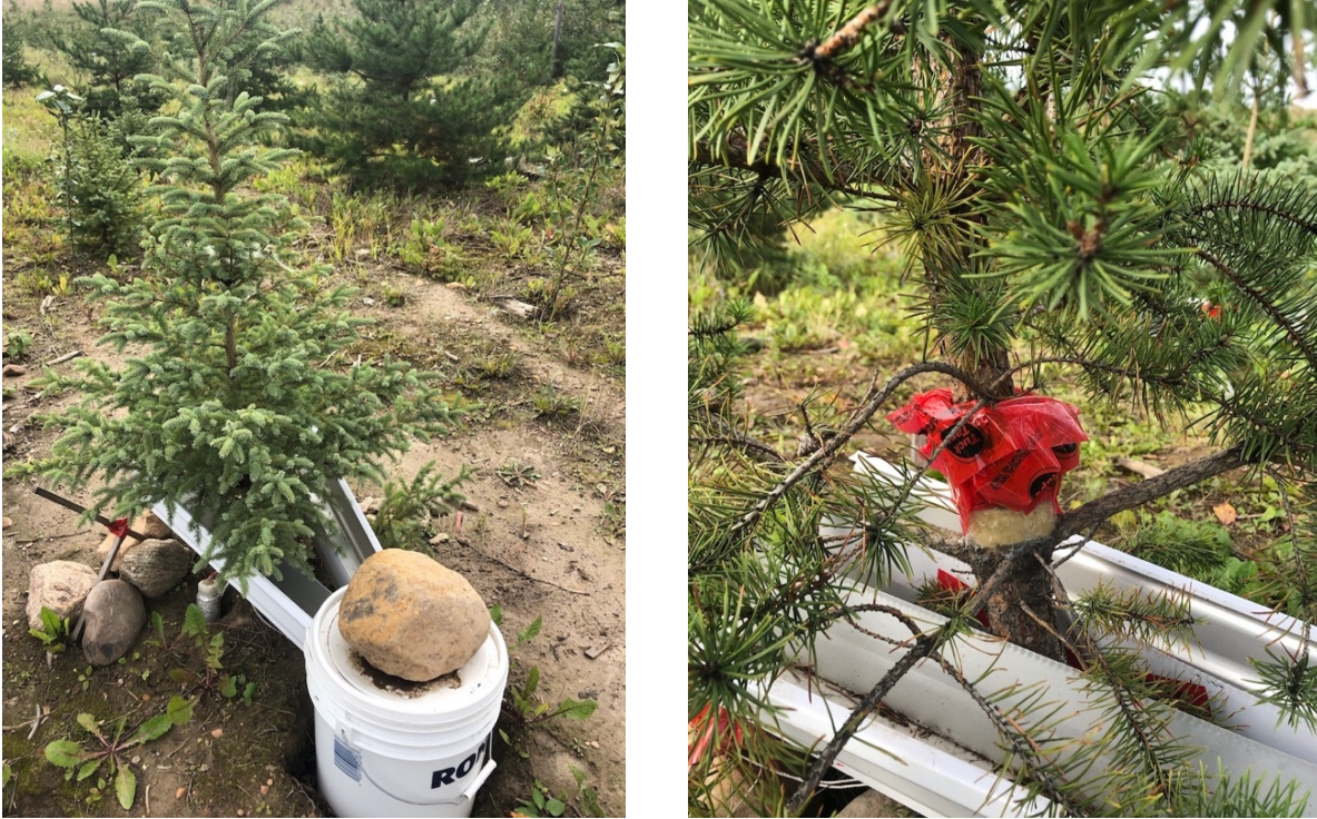
Figure 3: A) V-shaped throughfall collector capturing beneath canopy rainfall of an isolated Picea mariana tree, B) stemflow collector on an isolated Pinus banksiana tree.
