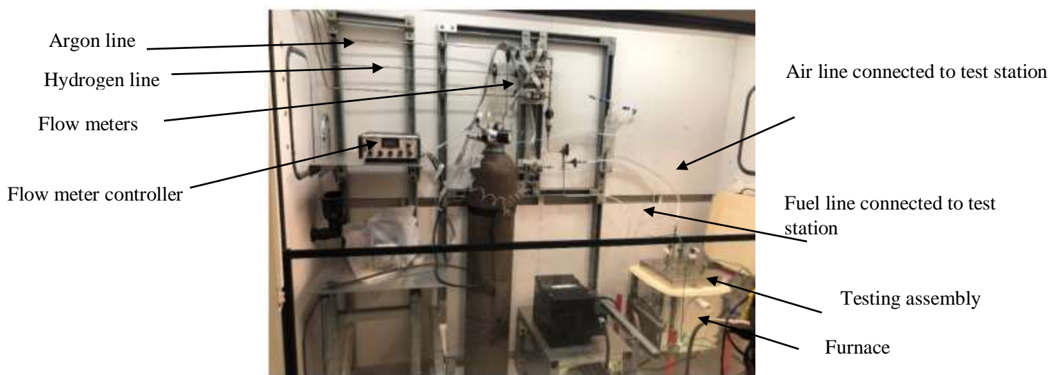
Figure 3.3 The test assembly with gas manifold inside the fumehood.
