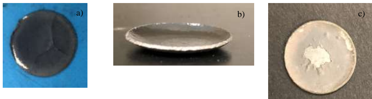
Figure 4.12 – Additional stand-alone cathode layer cell structures; a) more graded MS layer to anode transition layer, b) Cell co-sintered for 5 hours, c) Cell co-sintered for 4 hours.
