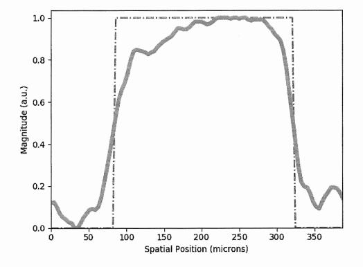
Figure 12. Normalized magnitude of intensity scanned across positive region of USAF resolution test chart. Group 1, element 2.
