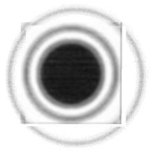
Figure 7. The centralized airy disc and its surrounding concentric airy patterns. Note how the airy patterns decrease in intensity the further they are from the airy disc.
