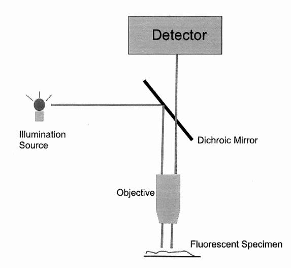
Figure 1. A diagram of a simplified fluorescent microscope. The blue ray represents the illumination or excitation light. The blue ray is directed towards the objective where it is focused onto the specimen. The emitted red ray is captured by the objective and passes the dichroic mirror and onto a photodetector.
