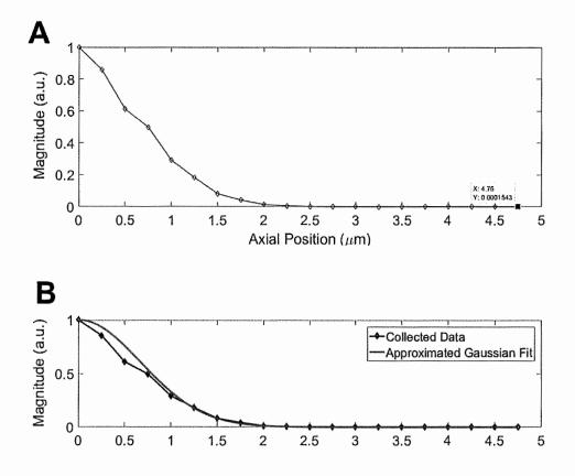
Figure 11. (A) Graph of the normalized intensity vs axial position of the mirror. (B) The normalized intensity compared to a Gaussian curve.
