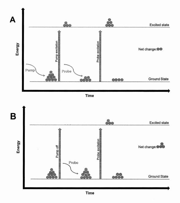
Figure 4. A schematic of an idealized two energy level diagram describing the transient absorption process. (A) The pump pulse drives some of the electrons to an excited state. The partially electron depleted ground state is probed and has less electrons to excite. (B) The pump is off and only the probe excites the electrons in the ground.
