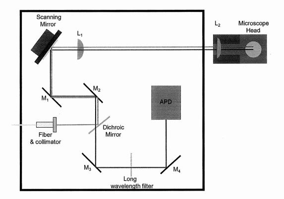
Figure 10. A schematic overhead diagram similar to figure 8, but without the spatial filter.
