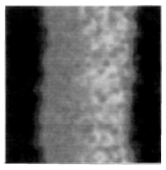
Figure 13. The image acquired from scanning positive region of USAF resolution test chart. Group 1, element 2.
