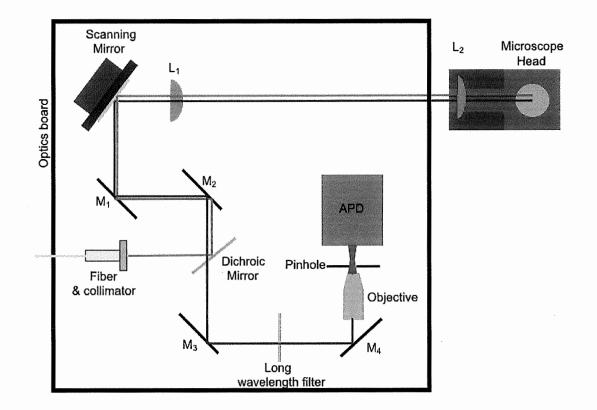
Figure 8. A schematic overhead diagram of the arrangement of the confocal optics. The circularized collimated beam (bright green ray) leaves the fiber and is directed towards the microscope head where it is directed downward and onto the sample. The dark green ray represents the emitted fluorescent light. It passes through the dichroic mirror and through the long wave length filter to ultimately be focused through the spatial filter and onto the APD.
