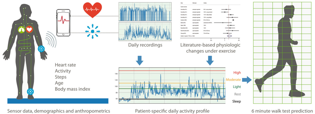
Fig. 5 Graphical summary. Step-by-step presentation of the concept for predicting 6-minute walk distances based on daily recordings from wrist-worn devices in combination with demographic and anthropometric data.
