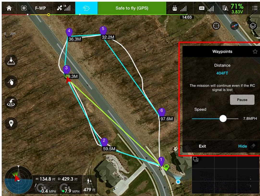
Figure A- 3: The operation window of DJI go for Phantom 3. Source: DJI
