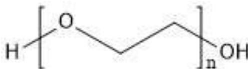
Figure 2.6: Chemical structure of PEG200.
