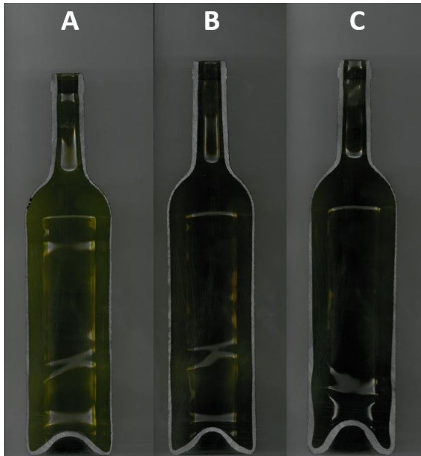
Figure 7 – Bottles A, B and C of increasing weight. Cut for wall thickness determination
