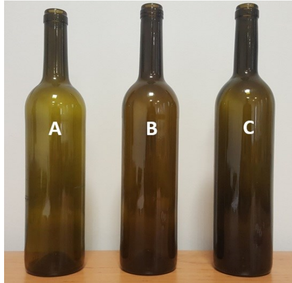
Figure 3 – Visually similar bottles identified in the study with different weights (Bottle A – 405 g, Bottle B – 458 g, Bottle C – 555 g)
