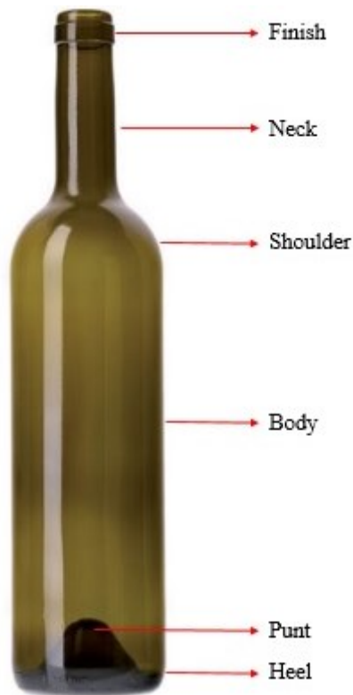
Figure 2 – Terminology of the different zones of a wine glass bottle
