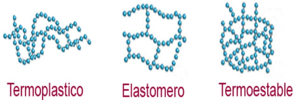
**Figura 3.** Estructura molecular CMP. [8]
