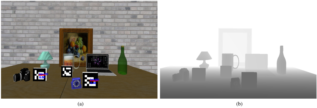
Fig. 10: Layout for the experiments with ordinary objects. a) RGB image of the scenario. b) Ground truth depth image
