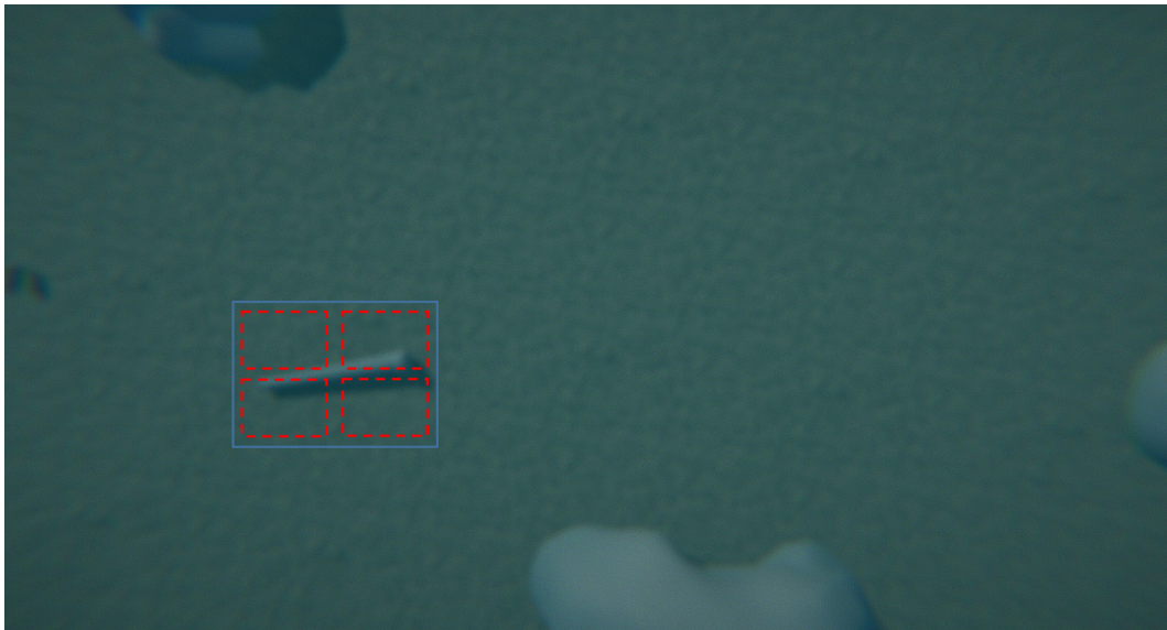
Figure 21. Vision phase 1: object identification (automatic or provided by the user).
