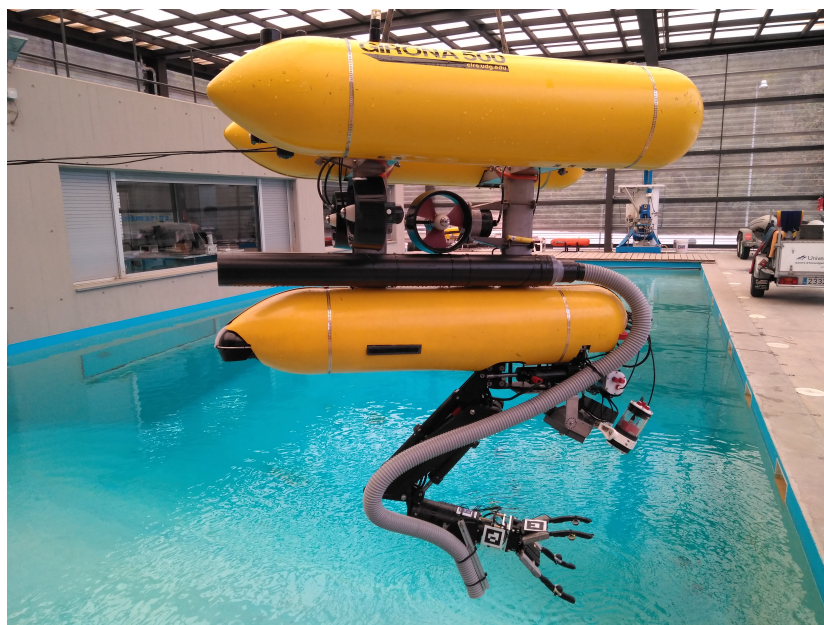
Figure 3. The Girona 500 and UJI Arm5E manipulator with tactile capabilities (image taken during previous MERBOTS project at the Research Centre in Underwater Robotics (CIRS) lab).
