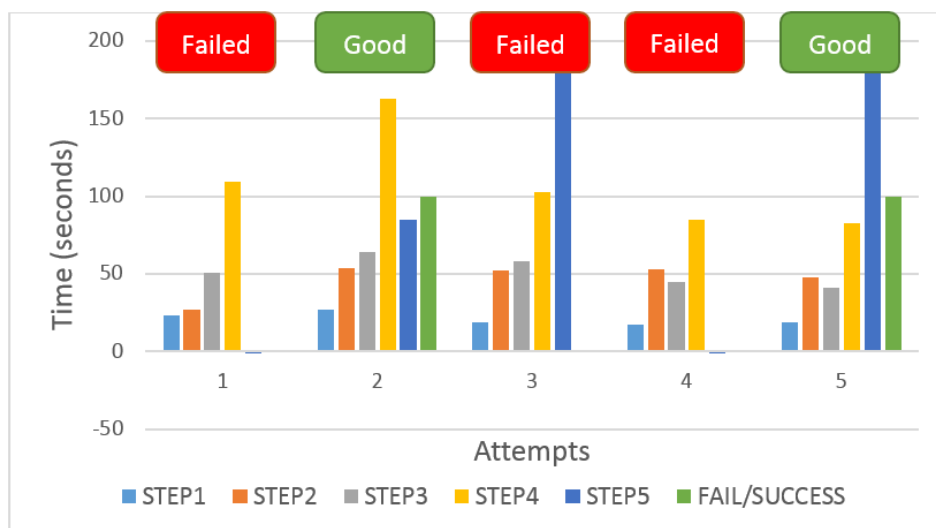
Figure 18. Usability test using 2 operators to teleoperate the team: 3 experiments failed, and 2 succeeded. The failures are due to human operator training (Y axis represents the intervention time).
