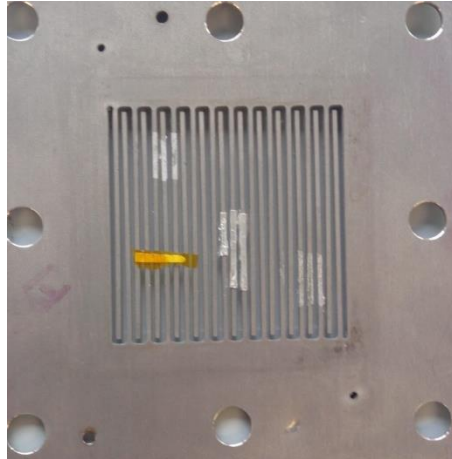
Figure 51: Aluminum foil in the ribs
