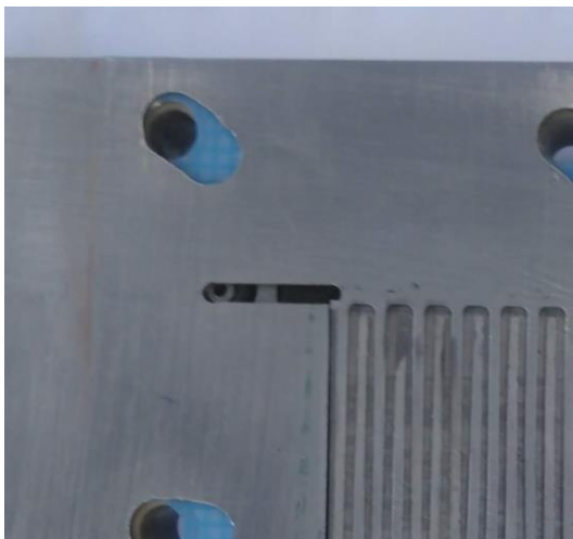
Figure 37: Close view from inlet and flowfield path
