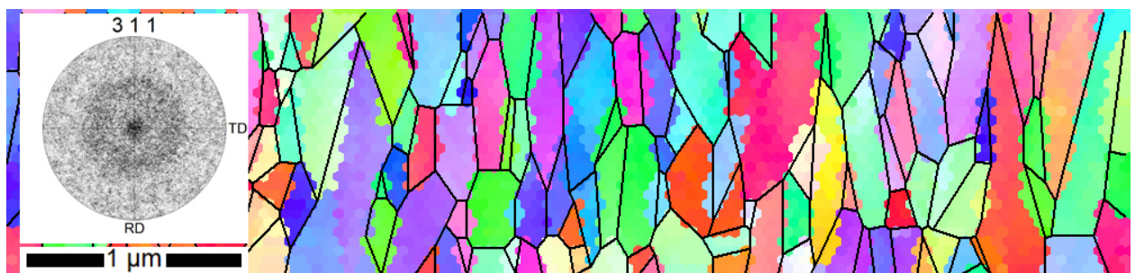
Fig. 4.16 - EBSD results for CrN layer of sample 1.1: unique grains colour map with reconstructed boundaries.
