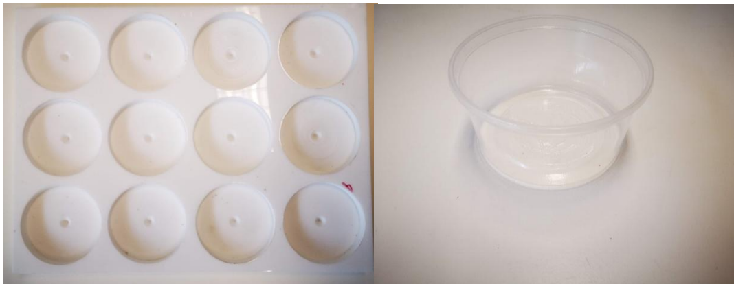
Figure 1 Types of arenas employed in the preliminary behavioral tests: a block of 12 arenas of 5 cm in diameter each (left) and the isolated arenas of 8 cm in diameter each (right).
