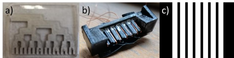
Figure 29. Silver electrode implementation. a) PDMS encoder; b) Reader; c) Pattern to be integrated at the encoder
