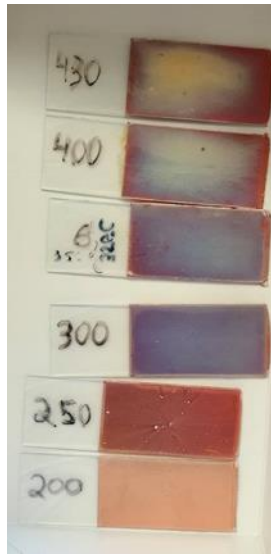
Figure 18. PTFE sample with different annealing temperature
