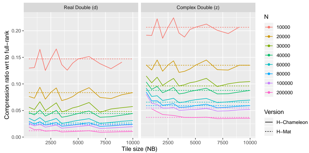
Figure 4: Comparison of the compression ratio between H-MAT-OSS original clustering algorithm (dashed line) and \mathcal{H} -CHAMELEON (full lines), in function of the tile size, for double precision (left) and complex precision (right).
