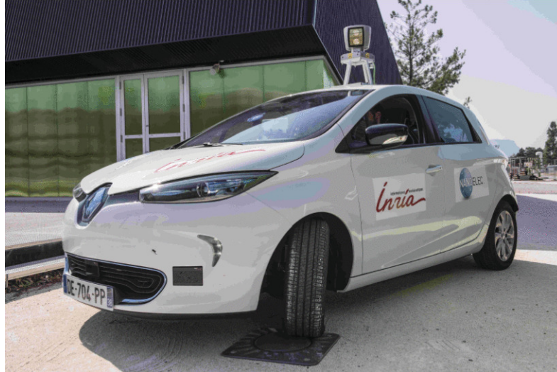
Fig. 8.2.: Renault Zoe instrumented platform used for capturing data used for evaluating the proposed algorithms. On the roof of this car is the velodyne used to record the dataset.
