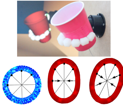
Figure 2.6: Examples of soft robots controlled via a real-time inverse problem based on FEM model, from Coevoet et al. (2019).
