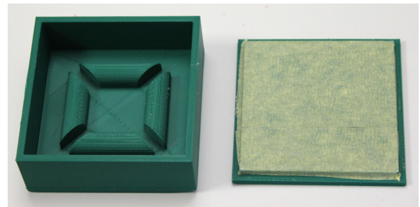
Fig. 3. An assembly of one of the two molds.
