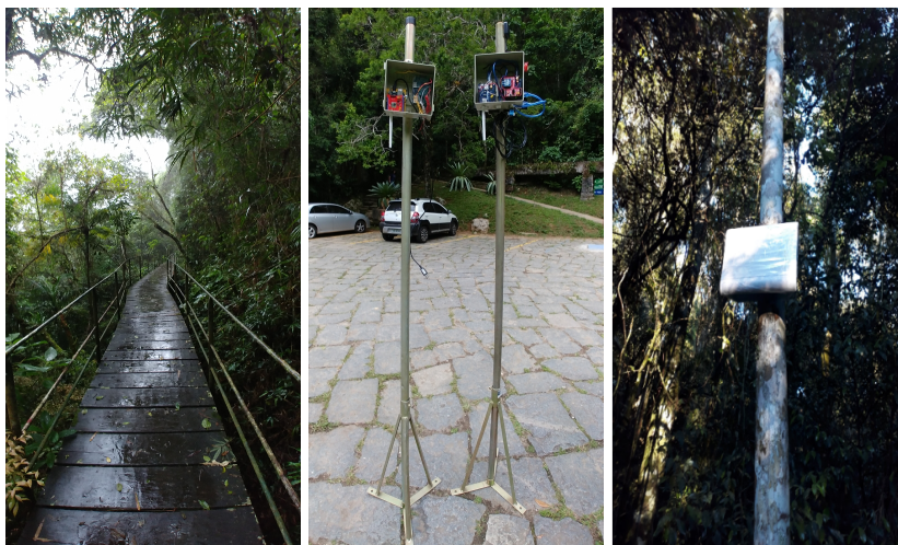
(a) The suspended trail. (b) Pole-mounted nodes. (c) Tree-mounted node.
