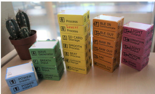
Figure 7: The created bricks, sorted by functionality. From left to right: power supplies, inputs (breathing, heart-rate, movement, ...), processing and merging, communication (analog, Bluetooth, serial, ...), and output (light, sound, vibration, ...).
