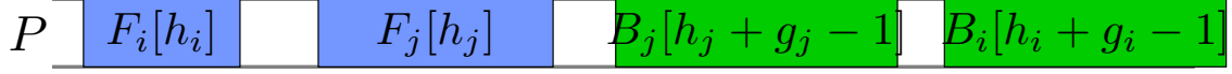
(a) Worst case. Memory needed to store the activations: g_i a_i + g_j a_j (reached between F_j and B_j ).
