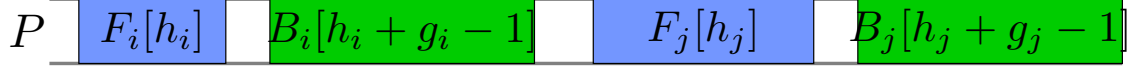
(b) Best case. Memory needed to store the activations: \max\{g_i a_i + (g_j - 1)a_j, (g_i - 1)a_i + g_j a_j\} (reached either after F_i or after F_j ).
