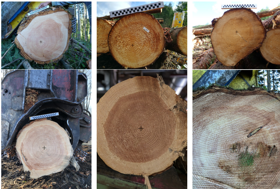
Fig. 5: Pith position (black cross) detected by the proposed method on raw log-end images using default parameters.
