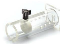
Figure 4.6. Mouse restrainer, 2’’ diameter tube with sliding nose restraint lock knob, ports and tail access for blood collection.
