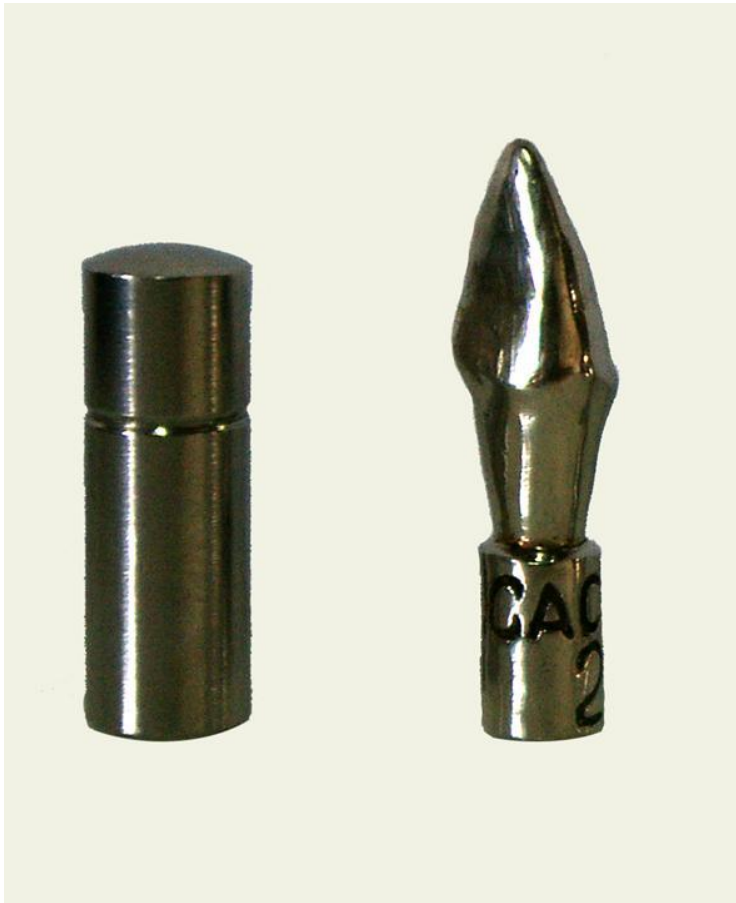
Standard Pentrometer head, and Cacajao prosthetic canine
