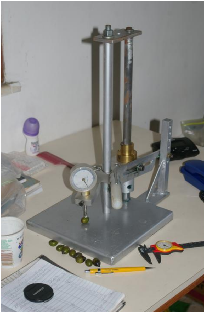
Test Rig, following the original Fridley Fruit Firmness Tester design of 1966
