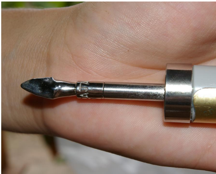
Prosthetic canine mounted on standard fruit penetrometer
