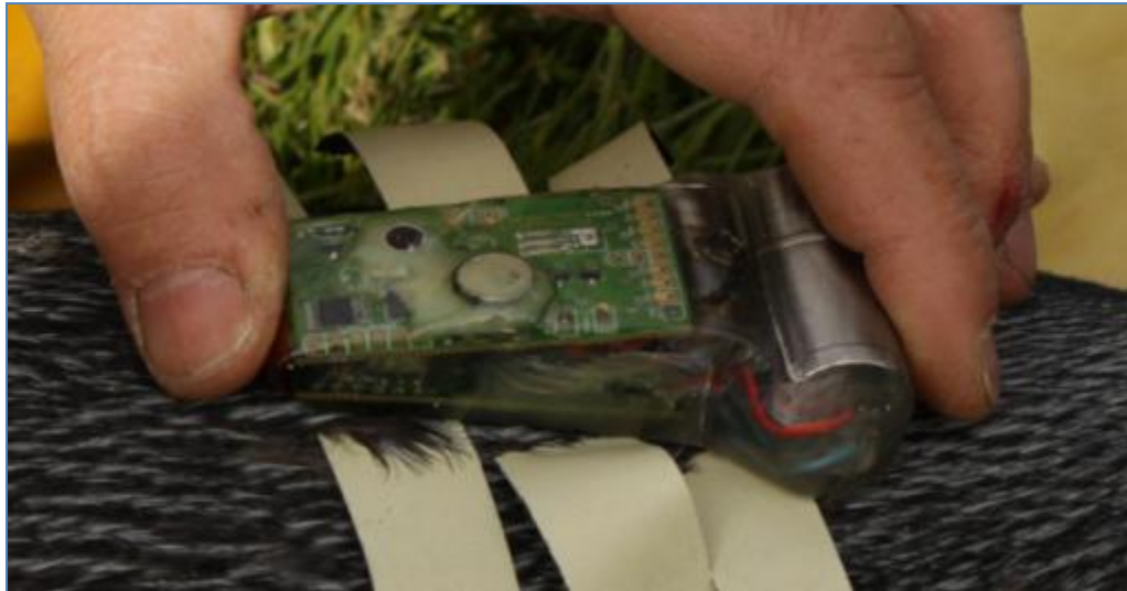
Figure 2.5 Accelerometer data logger being attached to a penguin.
