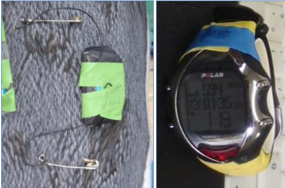
Figure 2.4 View of a Polar attached to a king penguin. Polar emitter (left) and a Polar receiver (right).
