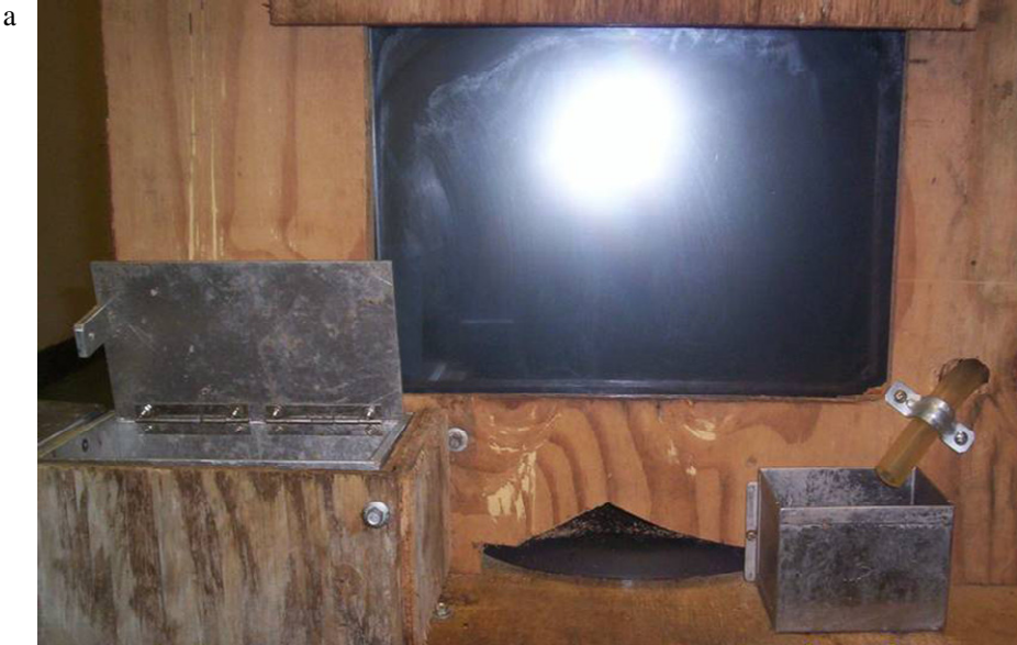
Figure 2.5 Laboratory apparatus. a) Touchscreen in wooden casing. b) Lunch box containing part of daily food ration. c) Pellet tray into which pellets are delivered from an automatic pellet dispenser via the plastic chute shown.
