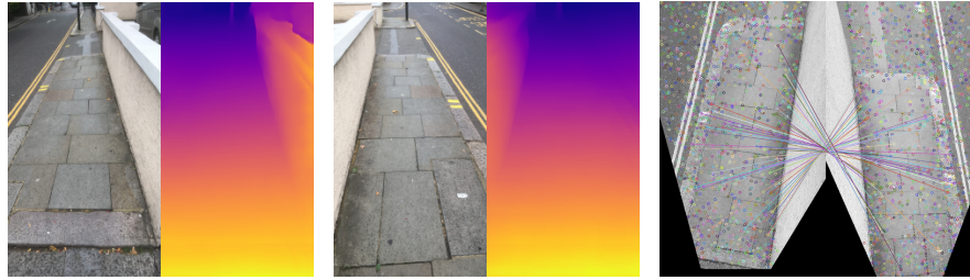
Fig. 1. Left to Right: Two input images, capturing the same section of a sidewalk, but looking in opposite directions. Each RGB input image is shown together with its depth map predicted by a single-image depth prediction network. Based on the predicted depth map, we identify planar regions and remove perspective distortion from them before extracting local features, thus enabling effective feature matching under strong viewpoint changes.
