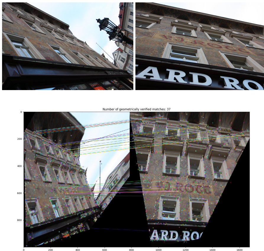
Fig. 11. Results on the Café scene in the EVD dataset. Top row: Original images. Bottom row: Geometrically consistent matches between the rectified patches.
