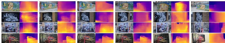
Fig. 4. “Failure” cases of applying a modern single-image depth prediction network [29, 74] on images from the HPatches dataset [6] (visualized as inverse depth): the network predicts the depth of the scenes depicted in the graffiti and images rather than understanding that these are drawings / photos attached to a planar surface.
