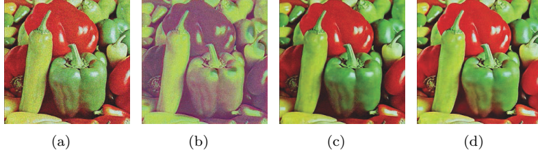
Figure 10: The denoising results with different loss functions. (a)noisy image, (b)denoised image with the adversarial loss (c)denoised image with the adversarial loss and pixel loss, (d)denoised image with the adversarial loss, pixel loss and feature loss.
