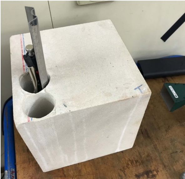
Fig. 2. Embedded material analysis of Darney sandstone (20x20x20cm) highlighting antenna position and insertion of obscured object. Antenna visible to the right of sandstone
