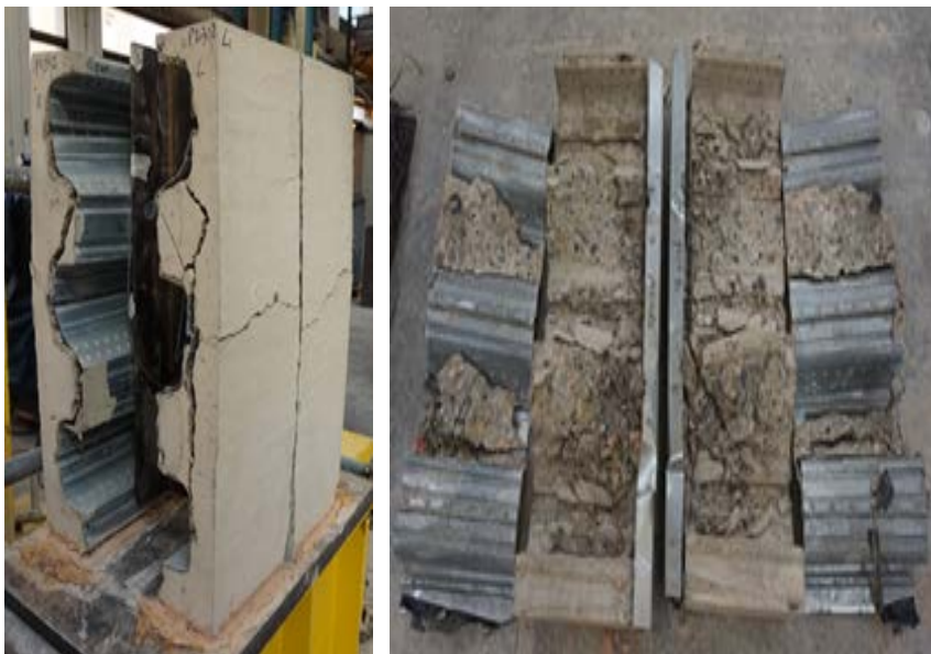
Figure 15: Specimen after the push test
