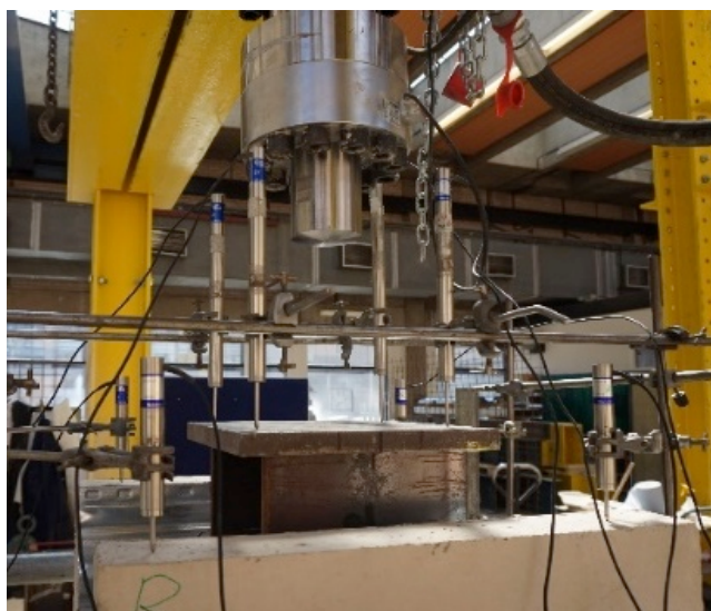
Figure 2: Positions of LVDTs
